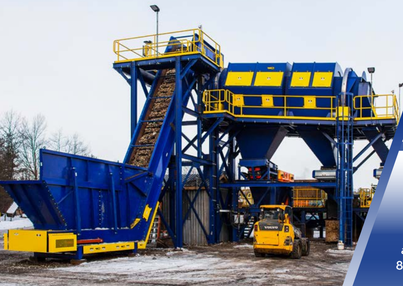
Integrated Batch Feeder Option with 5'x25' Trommel
