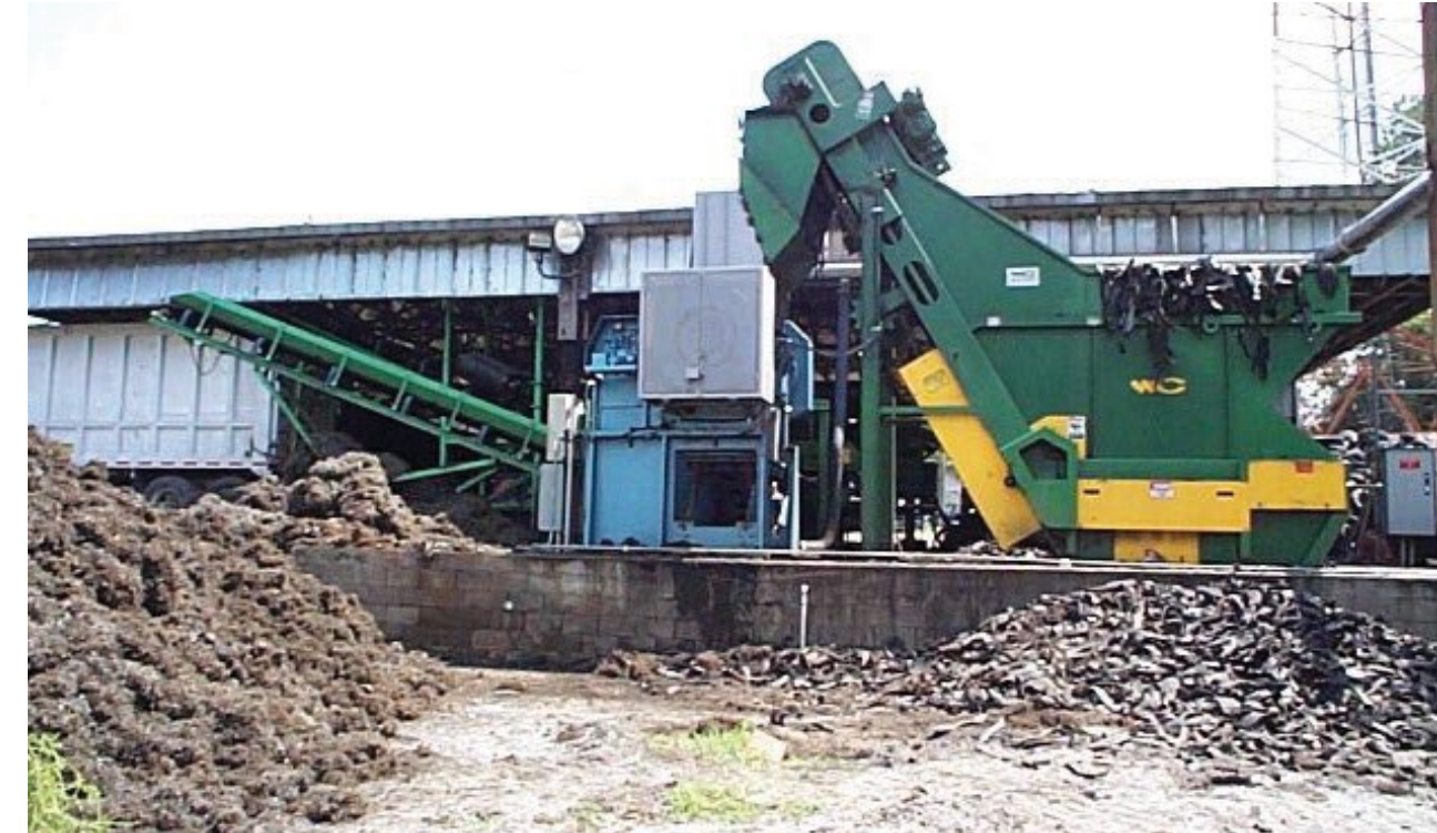
Typical Wendt Corporation Rasper installation at a tire recycling facility.
