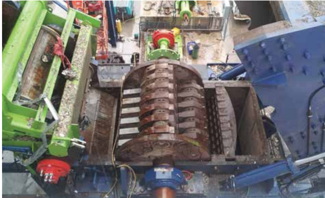
Top and bottom image: 8,000 hp Model 130 HEAVY shredder at EMR in Camden, NJ.
