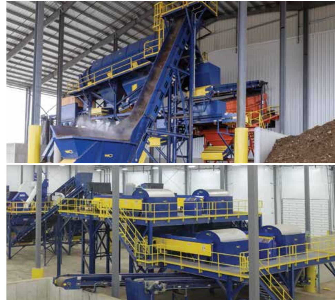
Sizing equipment preparing material for sorting (top image) and non-ferrous separation system installation (bottom image) at TJN Enterprises in Sioux Falls, SD.
