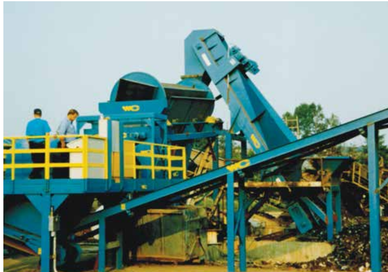
First EddySort system installed at Davis Industries in Lorton, VA, featuring the first Wendt TumbleBack Feeder and the first Wendt square screening trommel.
