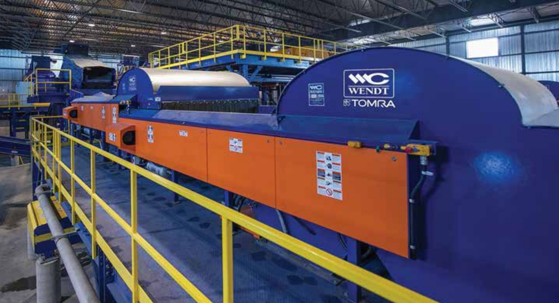
Non-ferrous separation and sorting system at Total Metal Recovery in Laval, Quebec, Canada.
